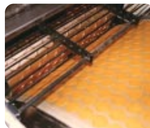
Rotary moulder application in a biscuit production line.
