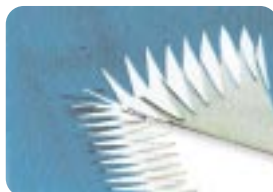
The durable jointing standard for multi-ply belts – double Z.
